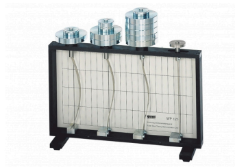
Demonstration of Euler Buckling
