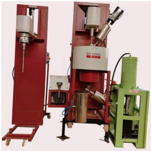
Bottom Pouring Type Stir Casting Furnance
