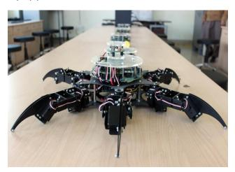
processors with 8 Gb of minimum RAM. Besides all the lab has other equipment like Robots which include FireBird V, Spark V and Hexapod. For embedded experiments the lab has INTEL Edison kits, sensors and other related devices. In the robotics lab students use a variety of robots, all specifically designed to serve a certain purpose, to either automate a task or assist the human technician/staff in completing a task.
