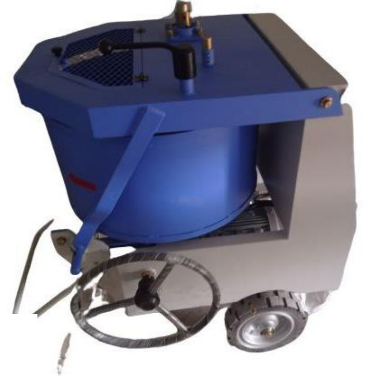
Pan Mixers Source: University Funds Purchase Cost: Rs. 1.66 Lakhs Concrete Lab
