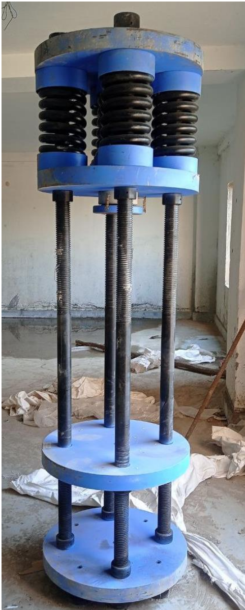
Creep test Rig Source: University Funds Purchase Cost: Rs. 3.50 Lakhs Highway Lab
