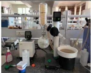
A Rotary Vacuum Evaporator (commonly known as a Rotavap) is a laboratory device used for the gentle and efficient removal of solvents from samples by evaporation under reduced pressure. It is especially useful for concentrating solutions or recovering solvents
