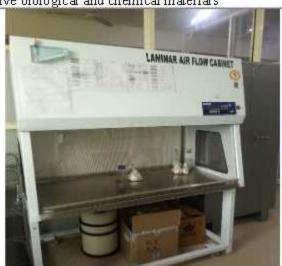
A Horizontal Laminar Air Flow Cabinet is a contamination-control device that provides a clean, particle-free working environment by directing HEPA-filtered air horizontally across the work surface. It is primarily used in laboratories for aseptic procedures that require a sterile and dust-free atmosphere.
