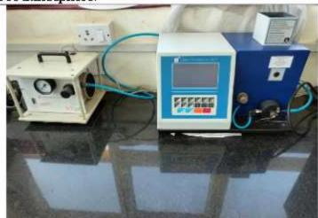
A Flame Photometer is an analytical instrument used to determine the concentration of specific metal ions—especially alkali and alkaline earth metals like sodium (Na<sup>+</sup>), potassium (K<sup>+</sup>), calcium (Ca<sup>2+</sup>), and lithium (Li<sup>+</sup>)—in a solution. It operates on the principle that metal ions emit light at characteristic wavelengths when introduced into a flame.
