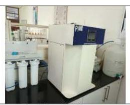
The Millipore Water Purification System is a high-quality laboratory system designed to produce ultrapure water (Type I) and pure water (Type II or III) for sensitive scientific applications. Manufactured by MilliporeSigma (part of Merck), these systems ensure the removal of ions, organics, particulates, bacteria, and pyrogens to meet strict analytical and biological requirements.
