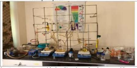
A Schlenk Line is a laboratory apparatus used for handling air- and moisture-sensitive chemicals under an inert atmosphere (typically nitrogen or argon) or under vacuum. It is essential in synthetic chemistry, particularly organometallic and coordination chemistry, where many reagents and products are highly reactive to oxygen or water
