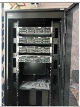
An HPC Cluster (High Performance Computing Cluster) is a powerful computing system that links multiple individual computers (nodes) to work together as a unified system for performing complex, large-scale computational tasks. It is designed to process, analyze, and simulate massive datasets or intricate calculations at high speeds, far beyond the capacity of standard desktop computers.
