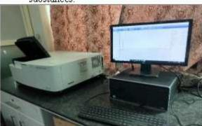
A fluorescence spectrophotometer (or spectrofluorometer) is an analytical instrument used to measure the fluorescence intensity emitted by a sample upon excitation with light of a specific wavelength. It is highly sensitive and suitable for detecting trace amounts of fluorescent molecules
