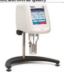
A **Brookfield Viscom eter** is a widely used instrument for measuring the **viscosity** of liquids and semi-solids. It operates by determining the **torque required to rotate a spin dle** at a constant speed in a fluid, which correlates directly to the fluid's resistance to flow
