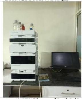
A High Performance Liquid Chromatograph (HPLC) is a powerful analytical instrument used to separate, identify, and quantify components in a mixture. It operates by passing a liquid sample through a column packed with a stationary phase, using a high-pressure pump to deliver the mobile phase
