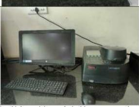
A UV-Visible spectrophotometer is a high-precision analytical instrument used to measure the absorbance or transmittance of light in the ultraviolet (200–400 nm) and visible (400–800 nm) regions of the electromagnetic spectrum. It is widely used in chemistry, biochemistry, environmental science, and pharmaceuticals for quantitative and qualitative analysis of substances.
