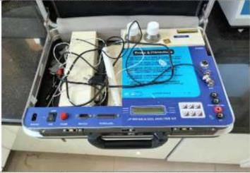
A Water and Soil Analyzer Kit is a portable, user-friendly analytical system designed for the rapid testing of key chemical parameters in water and soil samples. It is commonly used in environmental monitoring, agriculture, and field-based studies to assess nutrient levels, contamination, and overall quality
