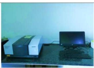
A Fourier Transform Infrared (FTIR) Spectrophotometer is an analytical instrument used to obtain an infrared spectrum of absorption or emission of a solid, liquid, or gas. It identifies and quantifies functional groups in organic and inorganic compounds by measuring how molecules absorb infrared light at different wavelengths
