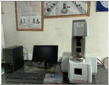
A rheometer is a scientific instrument used to measure the rheological properties of materials—specifically, how a substance flows and deforms under applied forces. It is essential for analyzing the viscosity, elasticity, and viscoelastic behavior of complex fluids and soft solids.
