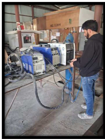
TIG & MIG WELDING SET UP
