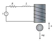
1. The system is at equilibrium (the ball is suspended in mid-air) whenever  $h = Ki^2/mg$  (at which point dh/dt = 0). Assuming the the following values for various parameters: m = 0.05kg, K = 0.0001, L = 0.01H,  $R = 1\Omega$ ,  $g = 9.81m/s^2$ , linearise the equations about the point h = 0.01 m i = 7 A and obtain the following linear state-space equations:
