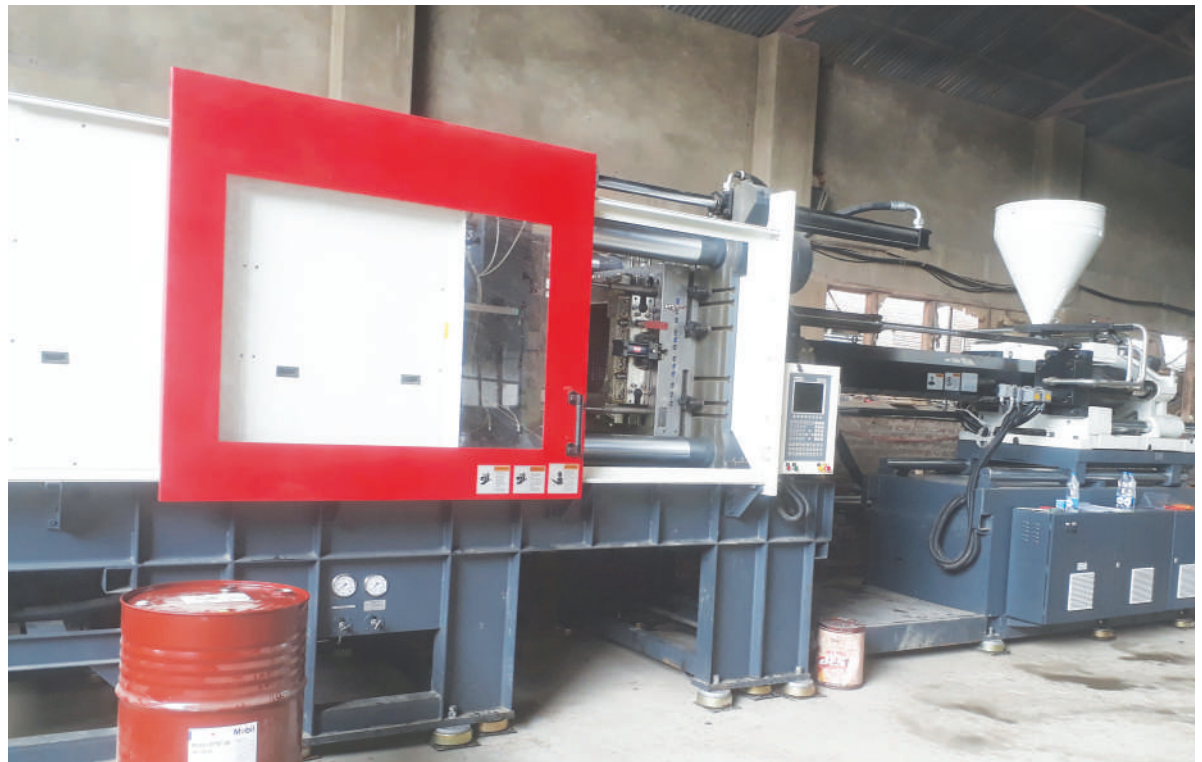
Plastic injection moulding machine in Supertherm factory at Shalteng industrial estate.
